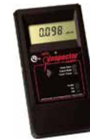
Inspector Survey Meter
